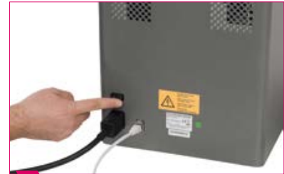
3 Turn on the main switch.
