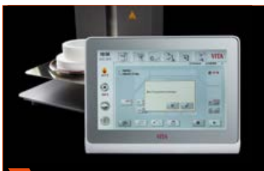
2 After opening the furnace, the message "Insert press material" appears.
