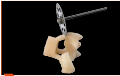
1 Separate press sprue with a thin diamond separating disc.
