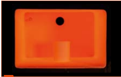
4 Place the investment ring in the furnace with the opening facing down. No contact with the furnace wall.
