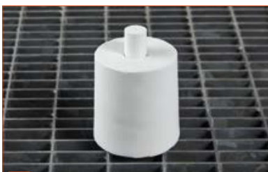
8 After removing the investment ring, allow it to cool in a protected place.
